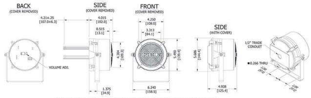
DIMENSIONS ARE IN INCHES [ mm ], TOLERANCES ARE IIO.03in [IIO.76mm] UNLESS OTHERWISE SPECIFIED.
